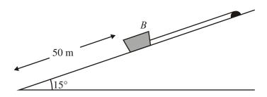
The diagram above shows a boat B of mass 400 kg held at rest on a slipway by a rope. The boat is modelled as a particle and the slipway as a rough plane inclined at  $15^{\circ}$  to the horizontal. The coefficient of friction between B and the slipway is 0.2. The rope is modelled as a light, inextensible string, parallel to a line of greatest slope of the plane. The boat is in equilibrium and on the point of sliding down the slipway.
